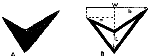
Fig. 1. (A) Drawing of typical AMPS spot illustrating the chevron or concave quadrilateral shape. (B) Calculation of the area of the spot in Fig. 1A: L is the base of both triangles, W is the sum of the two altitudes a and b and the sum of the area of the two triangles is \frac{1}{2} L \cdot W .
